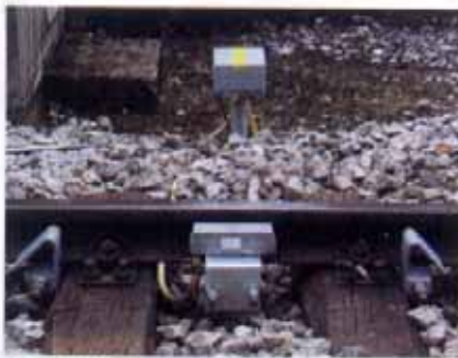
Fig. 2: ZK24 railwheel sensor
